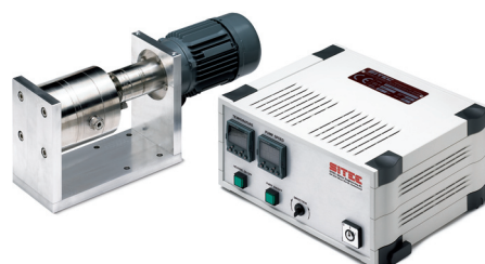
High-pressure gear pump for option «External recirculation» of upper and lower phase. It allows faster mixing of the phases or pulsation-free feeding to an injection loop for online concentration measurements (SFP, HPLC, etc.).
