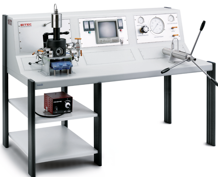
Phase equilibria unit with stirred optical cell and pressure-balanced piston for isobaric sampling. System includes also pressure generation, pressure and temperature control, colour camera with endoscope and cold-light source. Unit is in operation in a pharmaceutical company (Belgium).
